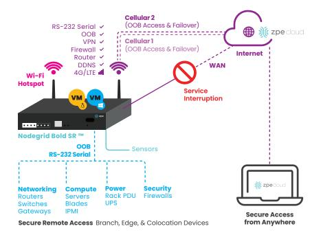
**Nodegrid Bold SR** is fast, secure, versatile and reliable. Bold in features and capabilities, **BSR supports a variety of connection methods:** serial, network, and USB. You get in-band and out-of-band remote access, power control, sensors and IT device health monitoring, alert notifications, actionable data, network backup, and more!
